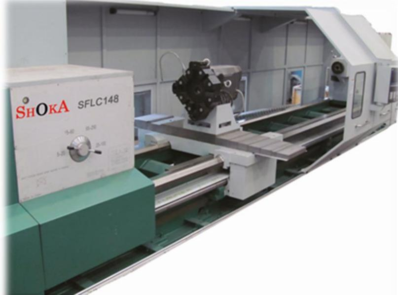
**CNC Flat Bed Lathe machine**
