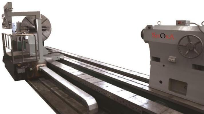
**CNC Flat Bed Lathe machine**
